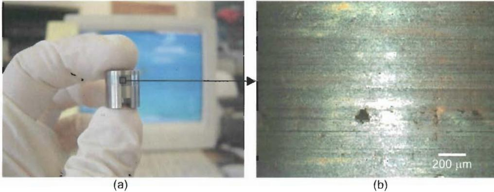
Figure 8. Images of tested roller after the test (4.4 millions contact cycles or 5 hours), in which ZnDTP was added after short test period with PAO only, (a) general appearance shows shiny, bluish surface of wear track, (b) microscopic image shows no micropitting with smooth surface.
