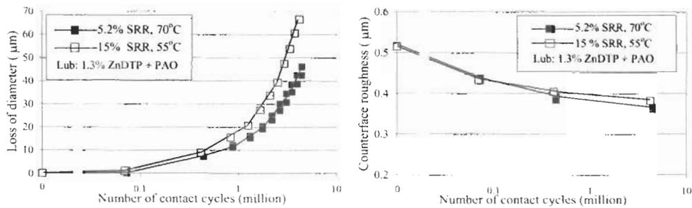
Figure 7. Effect of slide-roll ratio ( $\Delta v/\bar{v}$ ) on micropitting, (a) resulting wear curve, (b) variation of counterface transverse roughness ( $R_a$ )
