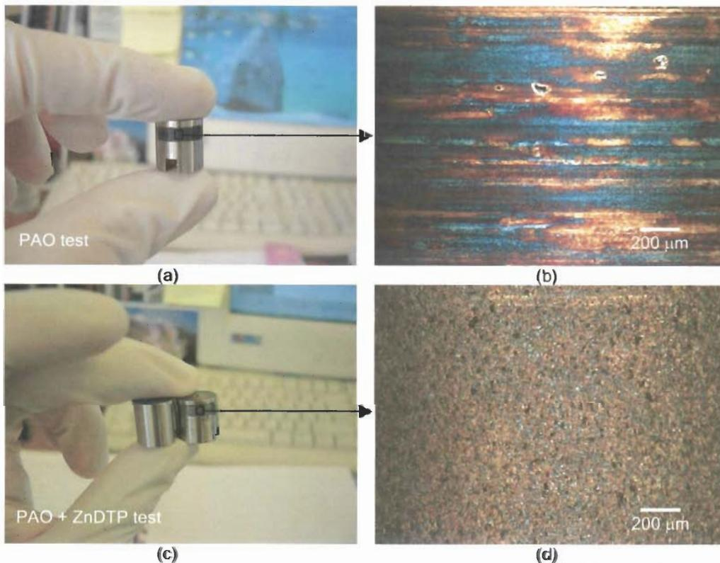
Figure 5. Images of the tested roller after 4.4 millions contact cycles (5 hours), (a) general appearance from PAO test, (b) microscopic image shows no micropitting, (c) general appearance from PAO + ZnDTP test compared with untested roller, (d) microscopic image shows micropitting covers the entire running track
