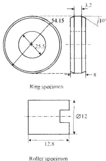
Figure 2. General geometries of ring and roller specimen (dimension in mm, not to scale)
