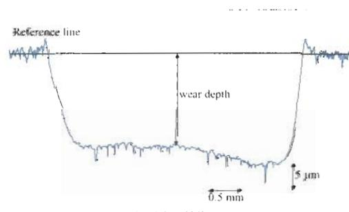
Figure 3. An example of worn surface profile, showing determination of effective wear depth
