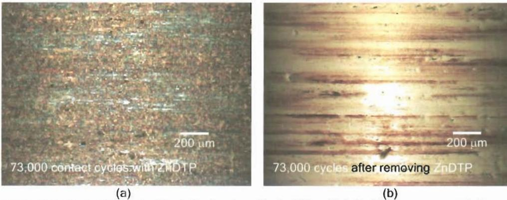
Figure 9. Microscopic images of tested roller from the test, in which ZnDTP was removed after short test period, (a) roller surface after short period test with ZnDTP illustrated an onset of micropitting, (b) roller surface after the same short period test following a removal of ZnDTP showed no micropitting with smooth surface.
