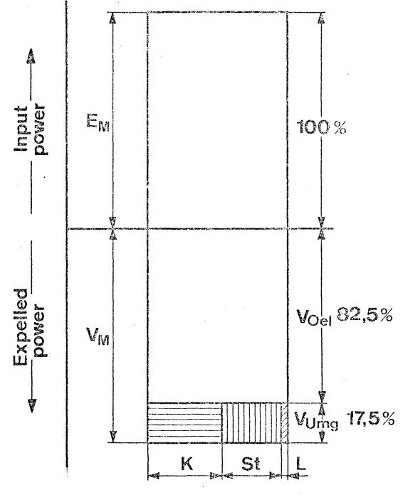
Heat dissipated into surroundings by K:convection St:radiation L:conduction
