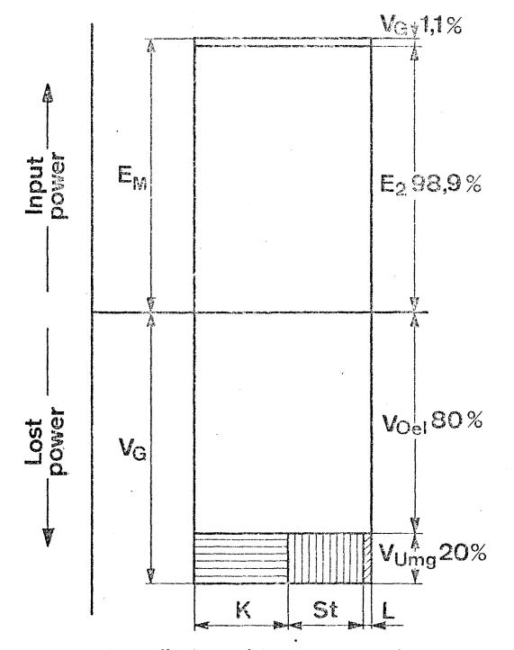
Heat dissipated into surroundings by K: convection St: radiation L: conduction
