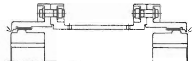
Figure 19. Spacer Coupling (Continuous Lube) with Reduced Overhung Moment on Connected Shafts, Most Common High Performance Gear Coupling in Use.
