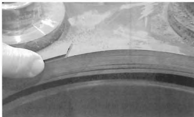
Figure 38. Outer Disc Failure.
