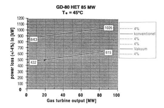
2. Determination of change in gearbox power loss under load. Gearbox power loss at full speed and increasing load can be assumed to progress linearly, because once full speed has been reached, only friction losses increase and the other loss factors (windage and churning) remain constant.
