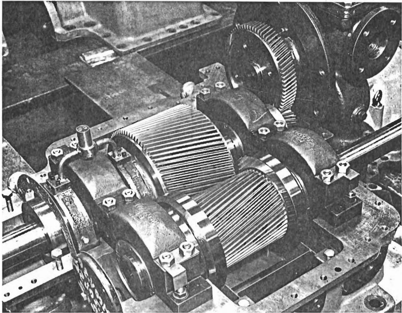
BST single helical precision gear between an LP and an HP compressor shaft. The BST thrust collar on the pinion takes up the axial gear thrust and, in addition, is used to transmit the thrust of the rigidly coupled high speed HP compressor shaft to the low speed wheel-shaft. With this technique, high speed toothed type couplings and high speed thrust bearings can be avoided which helps to improve decisively the reliability of the plant.
