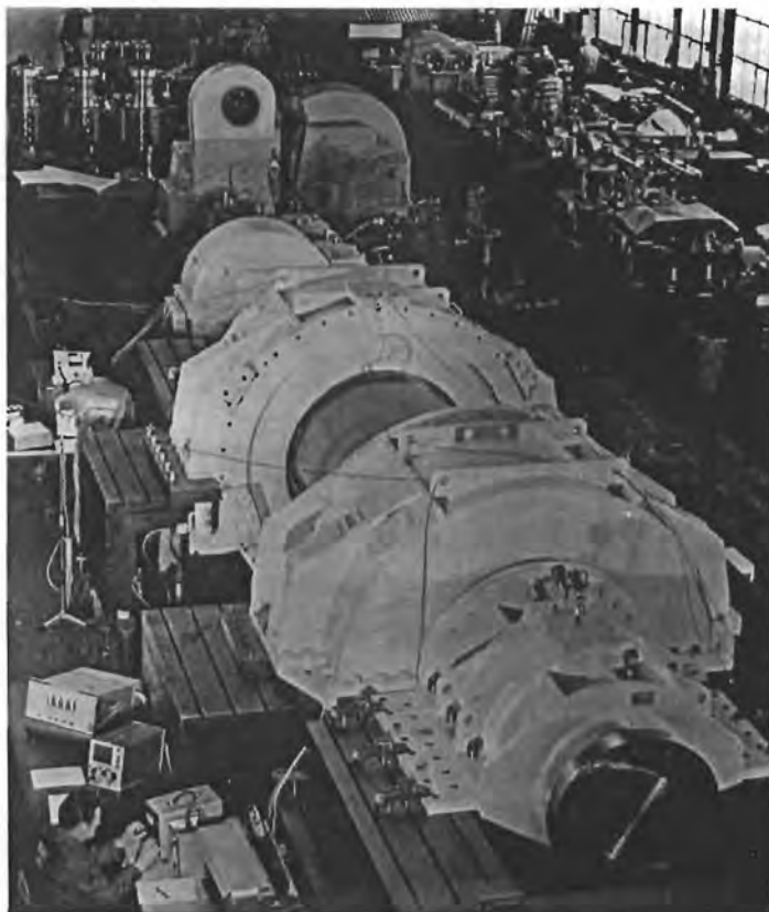
Fig. 11 Marine planetary gearbox on test rig. 13,200 kW, 400/122 rpm.
