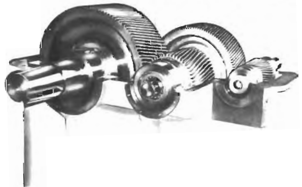
Figure 4. Two Stage, Single Helical Generator Drive Manufactured by American Lohmann. 4500 HP, 14500 RPM In, 1500 or 1800 RPM Out
