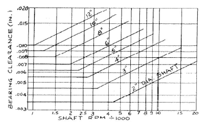
These values are based on 150 SSU @ 100'F oil with inlet temperature of 110'F to 120'F at 20 psig pressure. The above clearances are for standard bearings under normal operating conditions. Consult Artec for sizes and speeds not shown and special conditions. Tolerance +/-0.001" for 2"-6" diameters shafts +/- 0.015" for over 6" diameter shafts.
