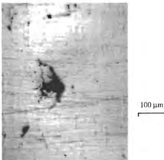
Fig. 2. Optical micrograph of isolated micropit used for the present study.
