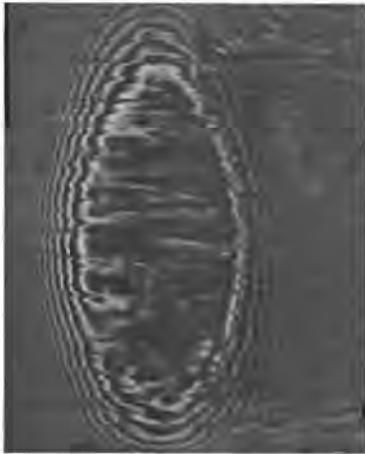
Fig. 10. Interference images showing micropit passing through contact under conditions of positive slide-roll ratio.
