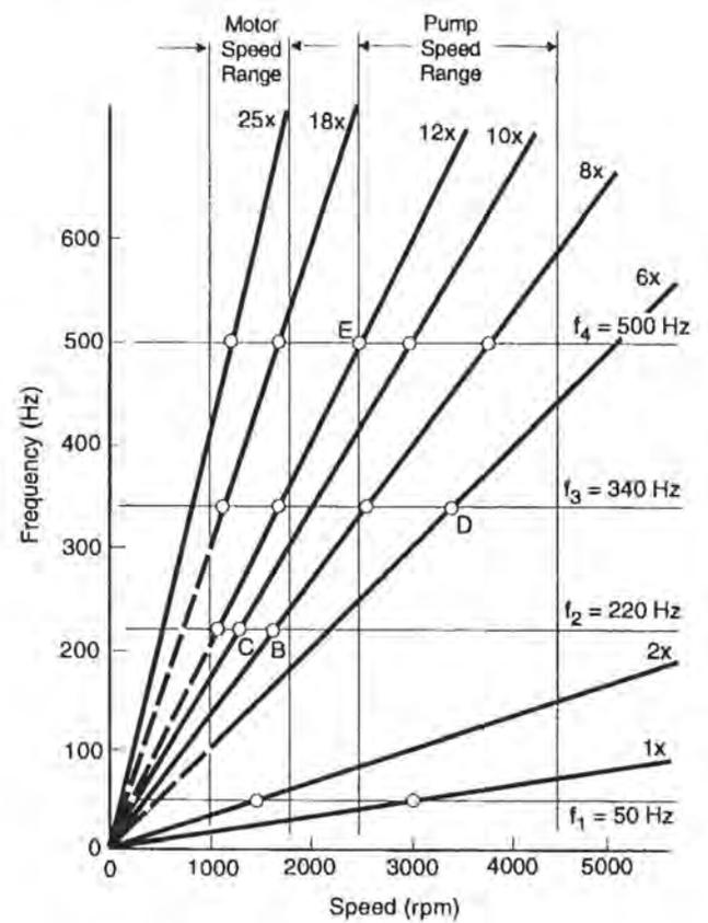
Figure 16. Combined Motor/Pump Campbell Diagram.
