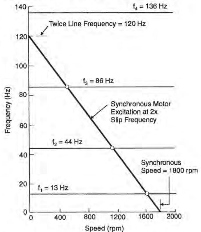
Figure 12. Synchronous Motor Campbell Diagram.
