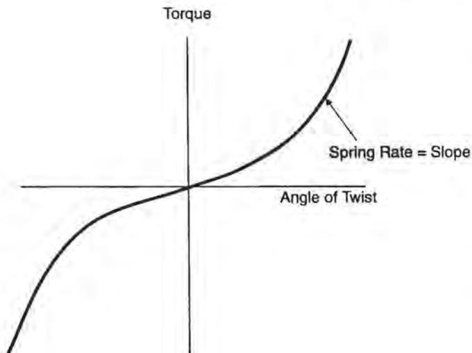
Figure 6. Nonlinear Coupling Behavior.
