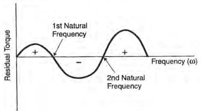
Figure 8. Residual Torque Behavior in Holzer's Method.
