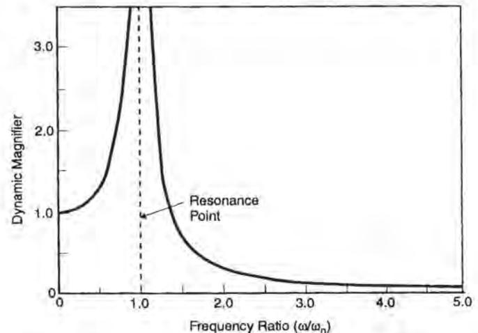
Figure 2. Undamped Response Curve for One D.O.F. System.
