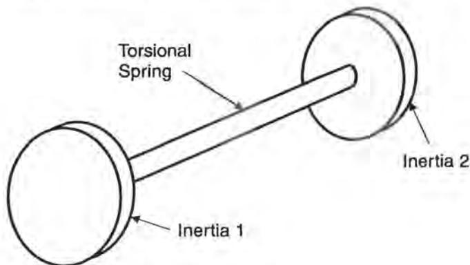
Figure 1. Two Inertia Torsional System.
