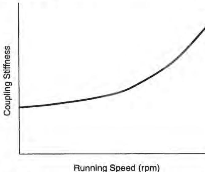
Figure 7. Nonlinear Coupling Stiffness Vs Speed Relationship.
