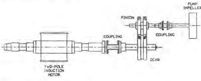
Figure 13. Example Motor-Driven Pump.
