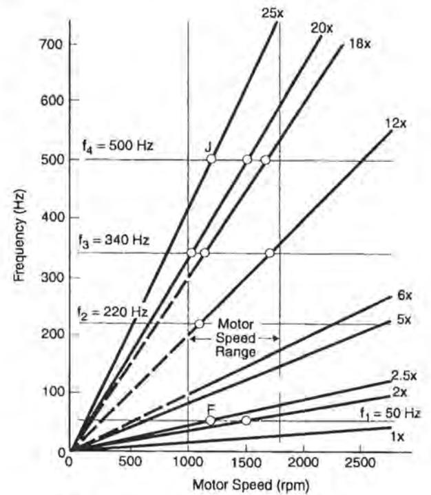
Figure 17. Combined Motor/Pump Campbell Diagram.
