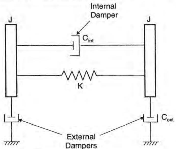
Figure 18. Modelling of Damping.
