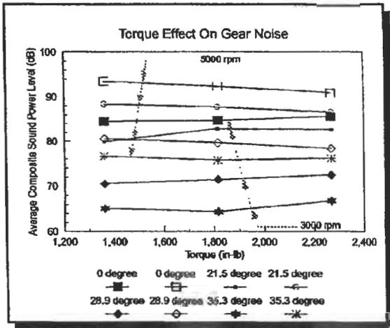
Figure 15 - Torque Effect On Gear Noise
