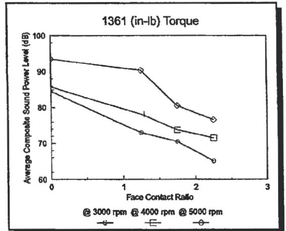
Figure 17 - Face Contact Ratio Effect Low Torque
