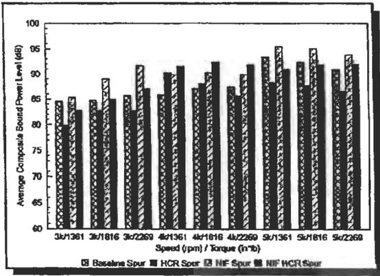
Figure 11 - Spur Gear Noise Levels
