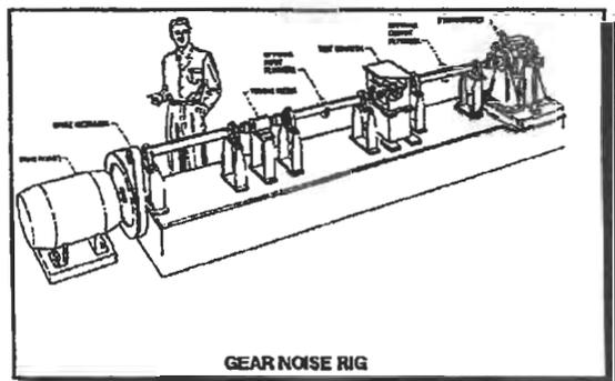
Figure 2 - Nasa Gear Test Rig
