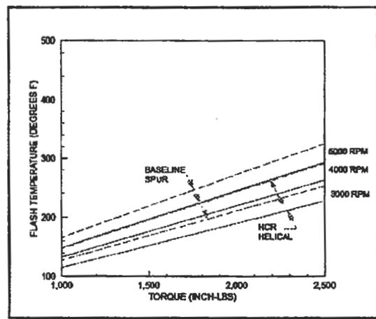
Figure 9 - Flash Temperature v Torque
