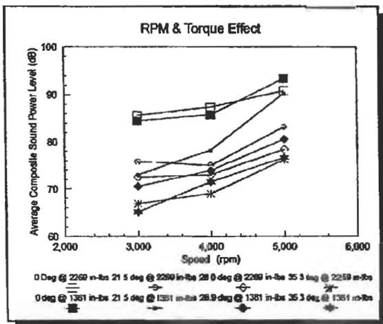
Figure 16 - Combined Speed & Torque Effects
