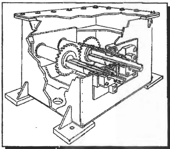
Figure 3 - Test Gear Box Cutaway Section
