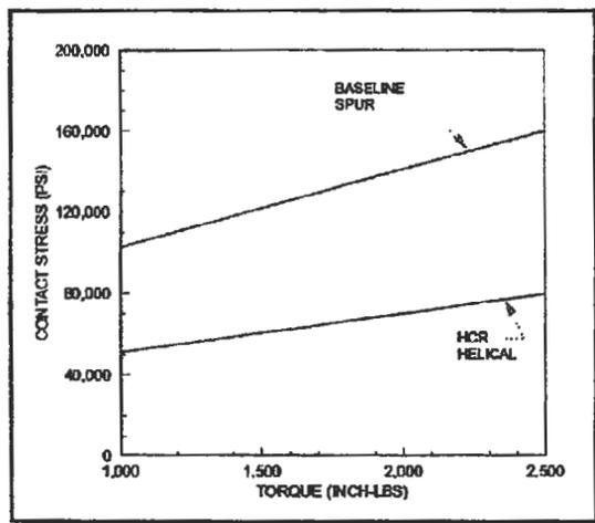
Figure 8 - Contact Stress v Torque
