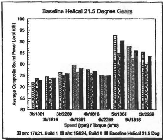
Figure 14 - Helical Gear Build Variations
