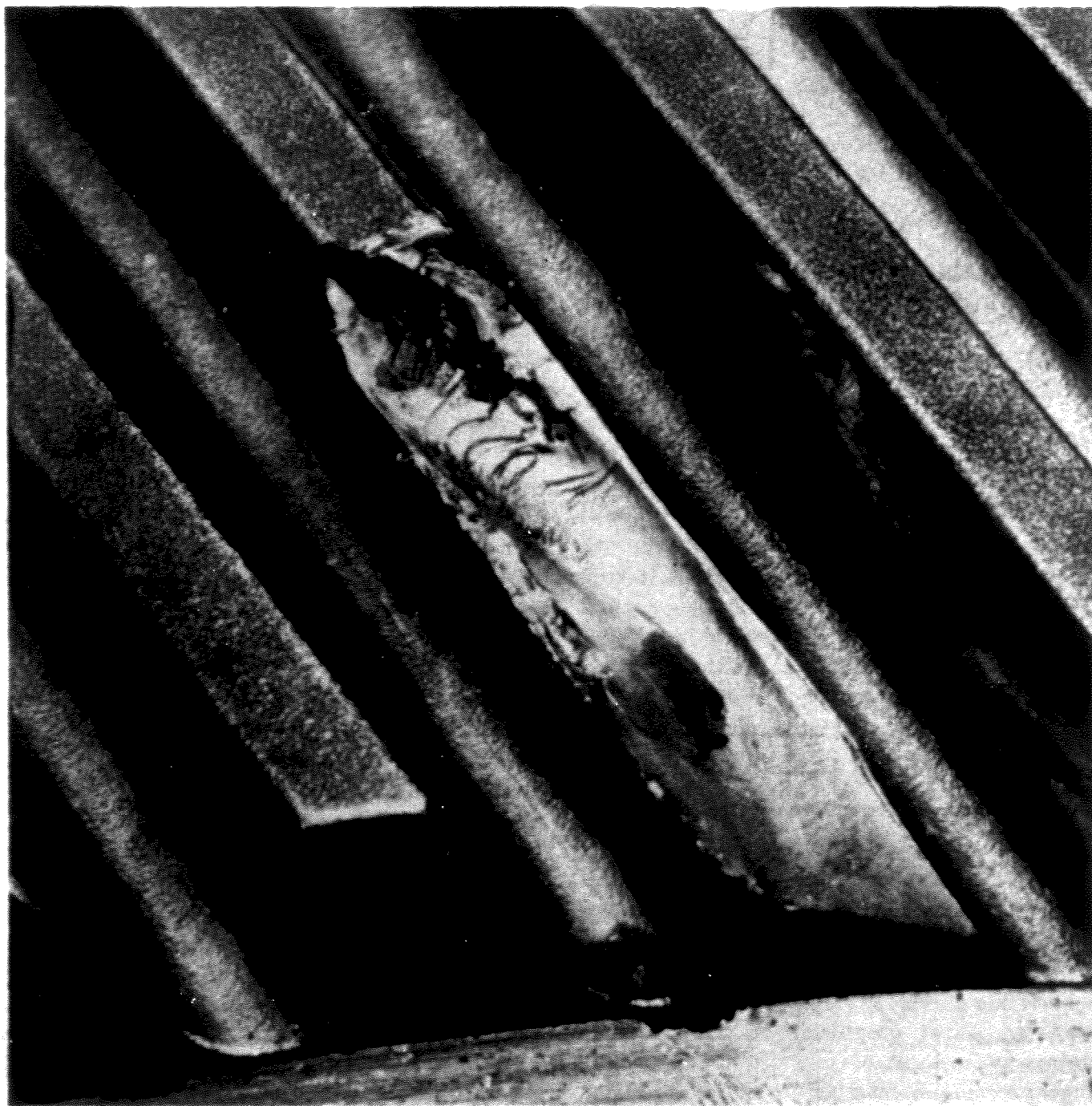
Fig. 25 Pinion tooth fracture—"B" unit
