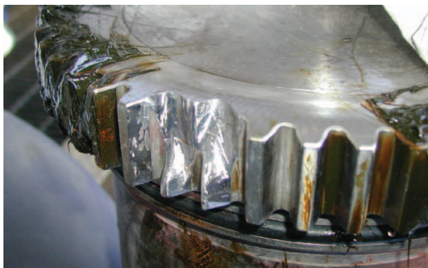
Figure 2. Refurbished gear tooth spacer ready to re-install as a temporary solution.
