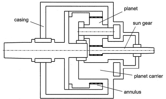
3: MAAG approach to a type PF turbo planetary gear unit
