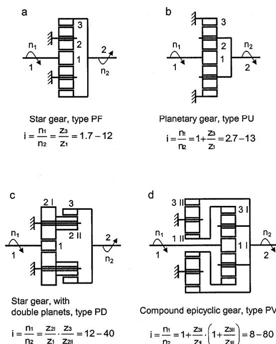
1: Turbo planetary gear unit variants
