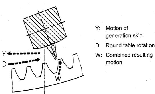
6: Principle of precision single-point tooth cutting as applied to internal gearing
