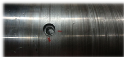
Precision removal of material to correct unbalance.
