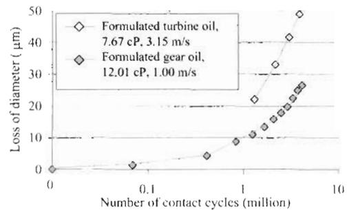
Figure 10. Wear curve from tests with two different formulated oils containing anti-wear additive. The viscosity given is corresponding to the inlet temperature for each test. The speed shown is the entrainment speed. Slide roll ratio was 5.2% in both cases.
