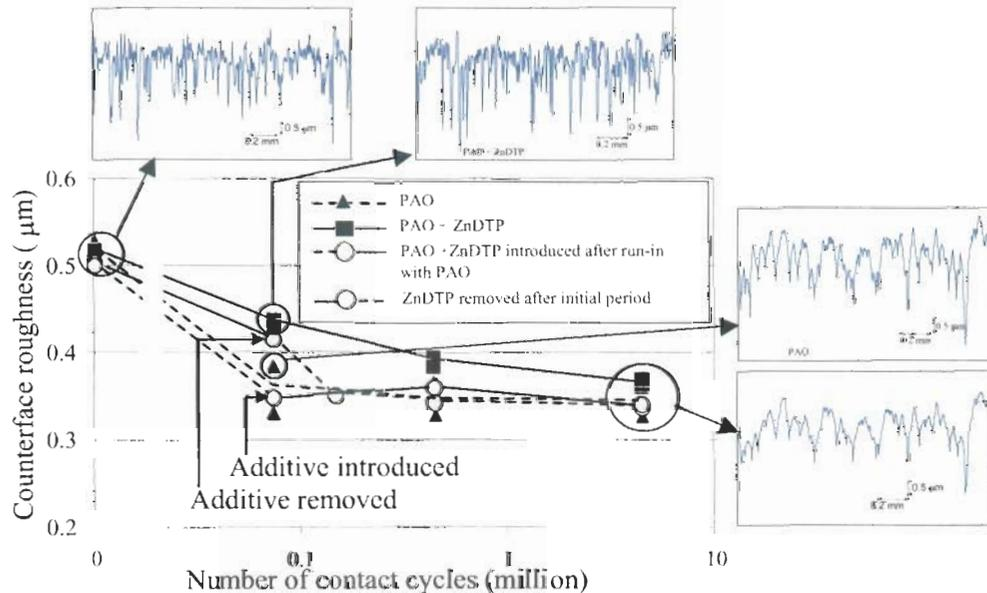
Figure 6. Variation of counterface transverse roughness ( $R_a$ ) during the test for PAO only and with ZnDTP tests. In general, the roughness of the counterface decline gradually during the test. Typical surface profiles before, during, and after the test are shown on the top and on the right hand side of the plot respectively.
