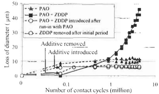
Figure 4. Evolution of wear as a function of contact cycles during the tests
